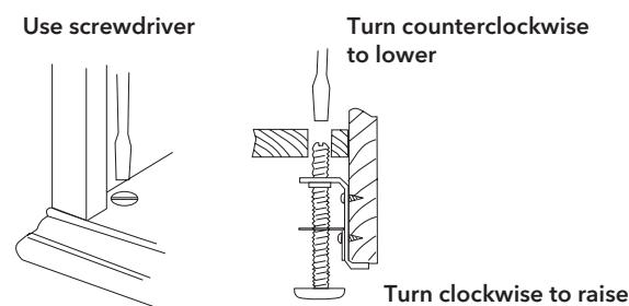
**External leveling.** When appropriate for the design of a unit, we include an external leveler, which is adjusted by hand. Once your furniture is in place, we recommend that one person tilt the case (or raise one corner slightly) to allow another person to adjust the leveler.
