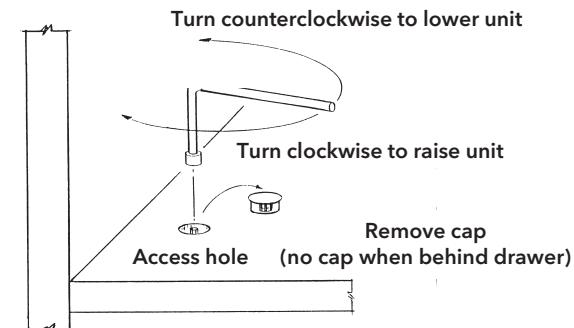
After alignment, replace the plastic cap.
